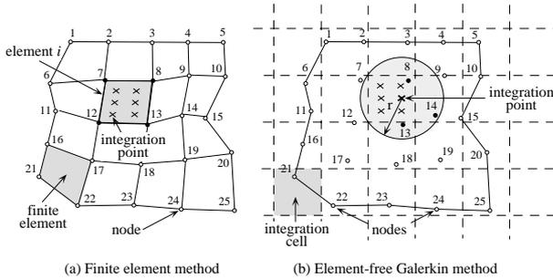
Fig. 1: Finite element method vs. Element-free Galerkin method
